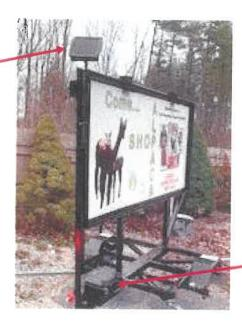
Case containing the light controller and 12 volt battery
