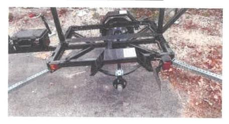
Once the safety legs have been extended and secured. Both the left and right tire/wheel will be removed from the portable sign to discourage theif. In addition, a pad-lock will be installed on the hitch.
