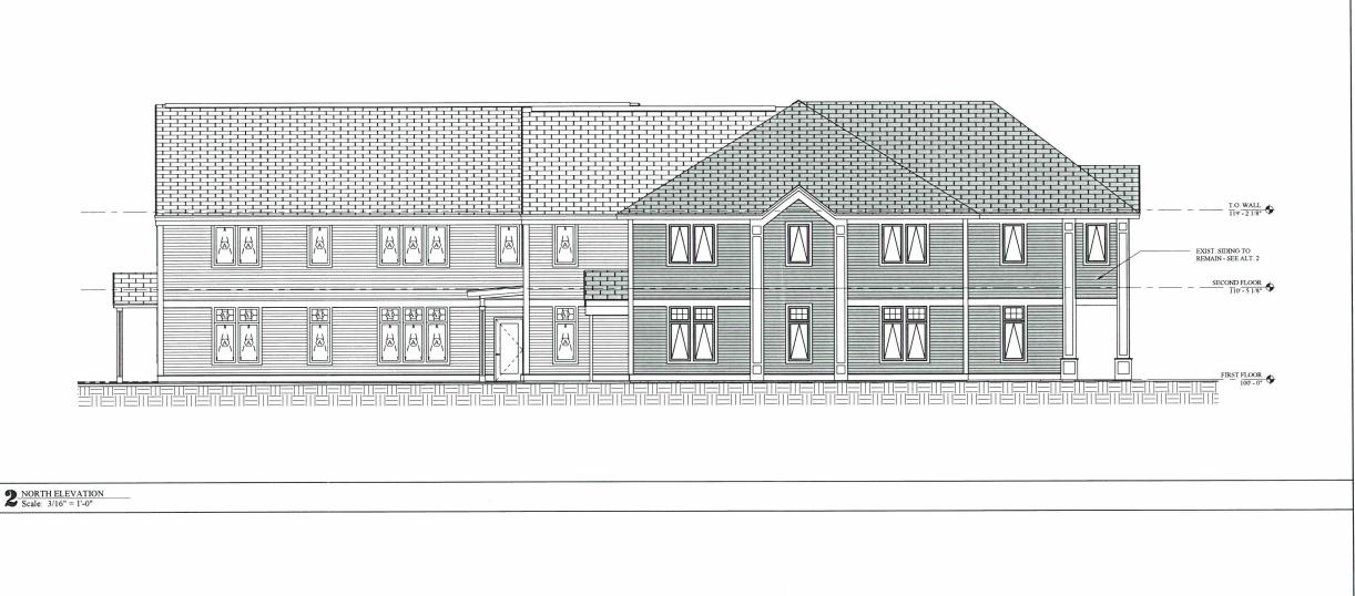
T.O. WALL 119' - 2 1/8" NEW WINDOWS BASED ON PELLA IMPERVIA NEW SIDING & TRIM TO MESH WE EXISTING UNLESS ALT. 2 IS ACCEPTED. NEW SHED ROOF
