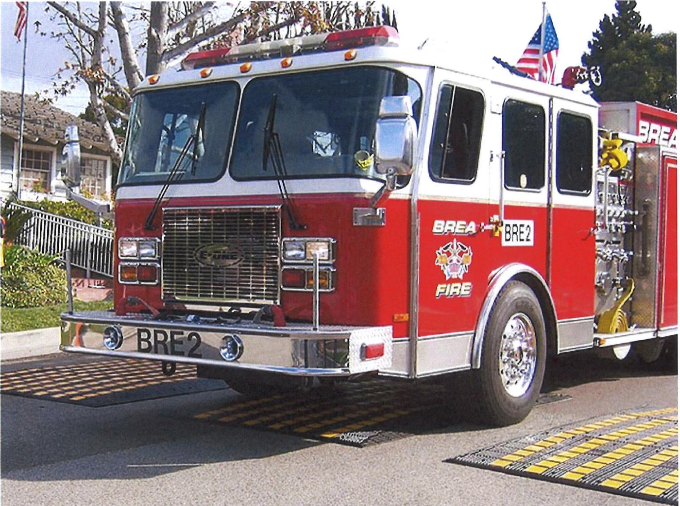
**Figure 5.1. Fire Engine Straddling Speed Cushion during a Trial Demonstration**
