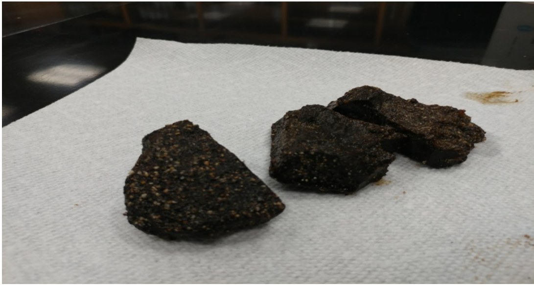
Sludge nuggets freed from the sand filter
